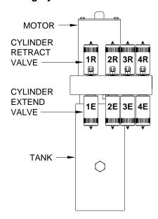
IMPORTANT: Open both the Cylinder Extend and Cylinder Retract valves for a room to release pressure before replacing one or both valves for that room. Turn the Valve Release Nuts NO MORE THAN 4 1/2 full turns counter clock wise to open the valves. Remember to close the valve(s) after the repair is complete. Tighten the Valve Release Nuts snug only. DO NOT over tighten.
