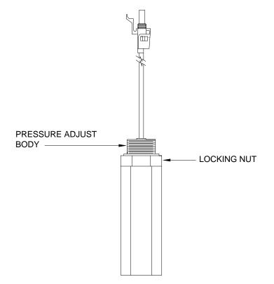
If the jacks or an individual jack comes down but does not touch the ground, do not adjust the level sensor. Adjust the pressure switch(es) as described above.
