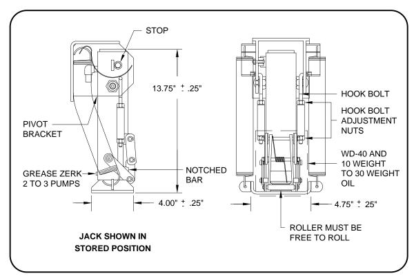
Regular lubrication is essential for the proper operation of this leveling jack.
