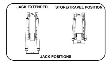
**CAUTION:** DO NOT MOVE THE VEHICLE WHILE ANY JACKS ARE EXTENDED. THIS VEHICLE IS EQUIPPED WITH STRAIGHT-ACTING JACKS. MOVING THE VEHICLE WITH THE JACKS EXTENDED CAN CAUSE SEVERE DAMAGE TO THE JACKS AND THE VEHICLE AND CAN CREATE A DRIVING HAZARD. DO NOT RELY SOLELY UPON THE WARNING LIGHTS, THE "JACKS DOWN" LIGHT, OR THE WARNING BUZZER AS AN INDICATION THAT ALL THE JACKS ARE IN THE STORE/TRAVEL POSITION.
