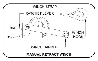
5. Slowly winch the room in by turning the WINCH HANDLE clockwise. The RATCHET LEVER should produce a loud, sharp, clicking noise.
