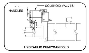
3. Open the SOLENOID VALVES by turning the "T" HANDLES counterclockwise.
