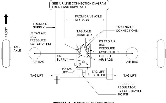
**IMPORTANT:** MANIFOLDS ARE PRE WIRED AND CONNECTIONS ARE LABELED. RIGHT AND LEFT CONNECTIONS MUST BE PROPERLY MAINTAINED
