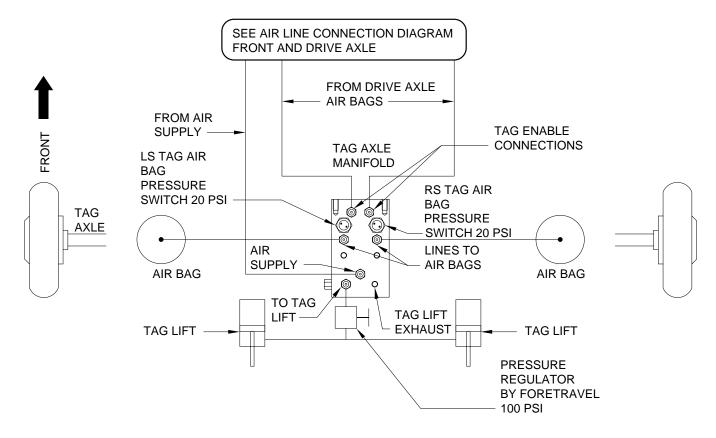
**IMPORTANT:** MANIFOLDS ARE PRE WIRED AND CONNECTIONS ARE LABELED. RIGHT AND LEFT CONNECTIONS MUST BE PROPERLY MAINTAINED
