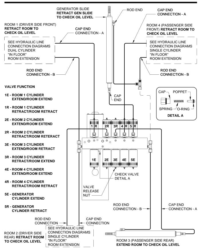
NOTE: HYDRAULIC PUMP SHOWN WITH ROOM EXTENSION MANIFOLD ONLY. THE LEVELING SYSTEM MANIFOLD (NOT SHOWN) IS MOUNTED ON TOP OF THE ROOM EXTENSION MANIFOLD.
