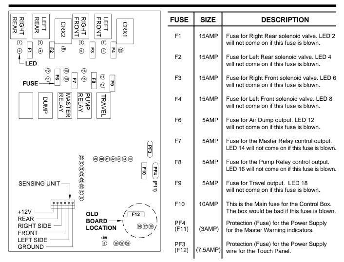
NOTE: On newer control boxes, FUSE F11 and FUSE F12 have been replaced with POLY SWITCHES PF4 and PF3. Poly switches protect a component or wire as a fuse does except the poly switch will allow current through when the overload or short is removed. Poly switches are not replaceable.
