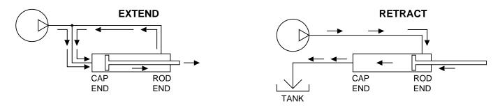
With a regenerative circuit, when extending the cylinder, there is essentually the same pressure on both sides of the piston. By making the area of the rod approximately ½ the area of the piston, we have approximately a 2:1 ratio of area size. This will give us equal force when extending and retracting the cylinder.
