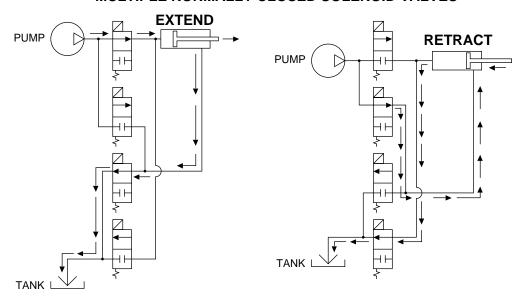
The regenerative circuit can be operated with two normally closed solenoid valves and a check valve. The check valve is used to keep oil from the rod side of the cylinder from flowing backwards to the pump when the pump is NOT running or when the pump pressure is lower than the rod pressure. This maintains the cylinder in the retracted position. There is also pressure on the rod side of the cylinder when the cylinder is extended but this is not critical for keeping the cylinder extended.
