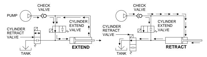
By using the regenerative circuit it allows the use of a simpler manifold with fewer valves. Fewer valves means less weight, less space needed [smaller manifold], fewer possible problems and reduced cost of the system. All of this makes the design of systems with multiple room extensions and slides more efficient.
