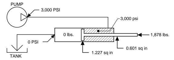
As you can see, by sizing the piston and rod size correctly, the force the cylinder in this example will produce is almost the same when extending, 1,803 lbs. and retracting, 1,878 lbs., moving the room out and in.
