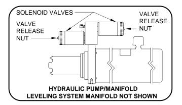
3. Open the Solenoid Valves by slowly turning the valve release nuts counter clockwise using the 1/4" nut driver supplied.
