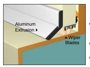
▲ The aluminum extrusion works as a "shovel" to remove larger debris while the wiper blades bend, similar to a "squeegee", to remove finer debris and water.
